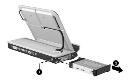
Removing the Hard Drive Carrier
